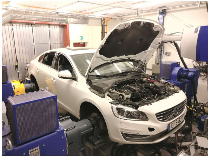
FIGURE 9: Test-bench setup. A conventional passenger vehicle is used with the same CE and EM as shown in Fig. 3.
