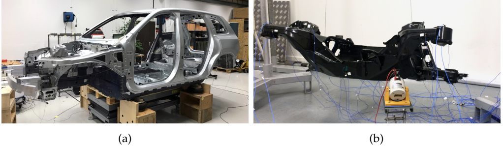
Figure 2.1: Experimental set-up of a BIW on air springs in (a) and rear subframe hanging in lines in (b).
