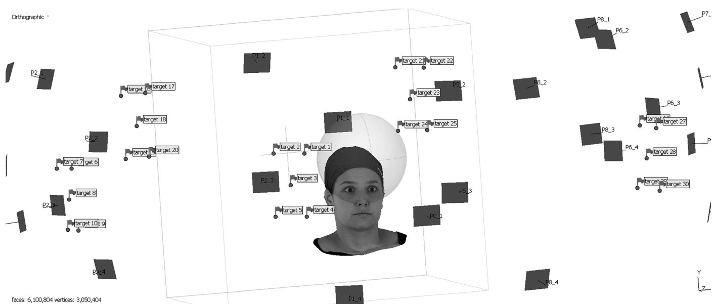
Figure 4: A CG face generated through photogrammetry by using 33 photos captured from different angles.
