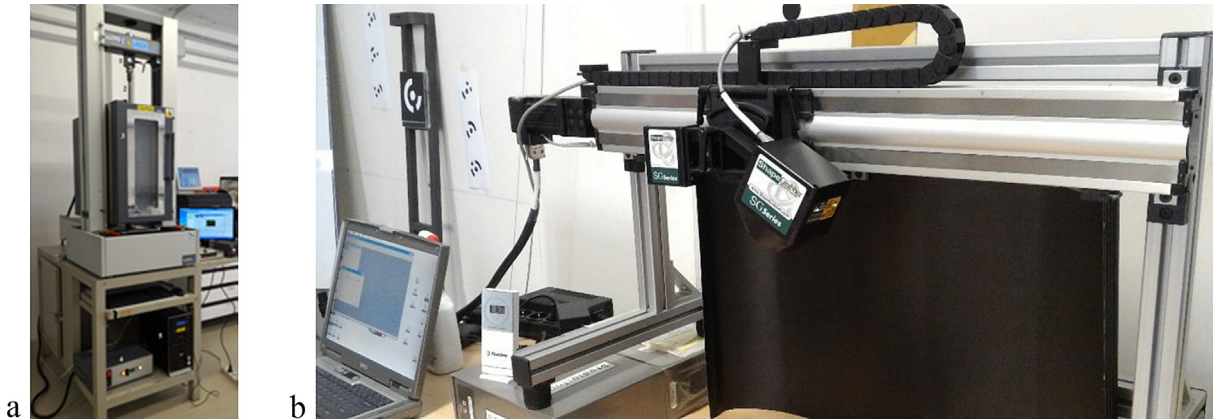
Fig. 4. (a) LLOYD Instruments LR50K Plus materials testing machine equipped with oven; (b) ShapeGrabber LM600 3D scanner Batch of two composite laminates.
