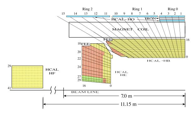
Figure 3.7.: The layout of the CMS HCAL (quarter slice), figure taken from [101]. The locations of the front end electronics is indicated by FEE, the rest of the calorimeter is split into the barrel region (HB), the endcap region (HE) and the forward region (HF). The outer detectors denoted with (HO) are located outside the magnet coil in order to catch the energy leakage from the HCAL barrel detectors.
