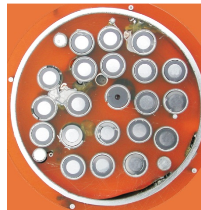
QUENCH-08: moderate melt formation; no noticeable melt relocation
