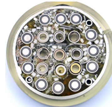
cross-section at 400 mm: metallography; debris bed porosity 50%
