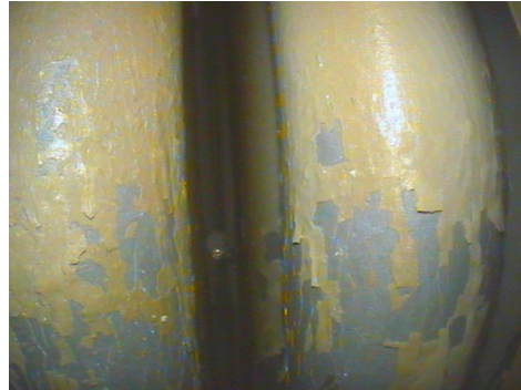
Endoscope observation at ~850 mm
