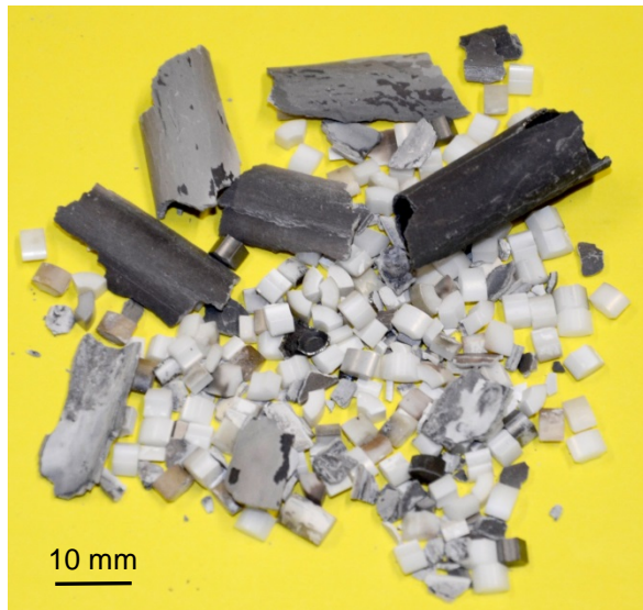
debris: 1) separated parts of fuel pellets simulator; 2) large segments of failed Zry claddings.
