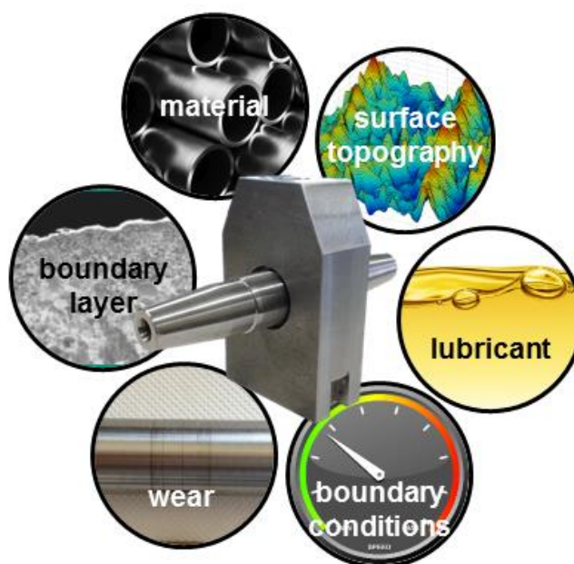
Figure 3-1: Influences of a tribological system on the demonstrator of a bearing and a shaft
