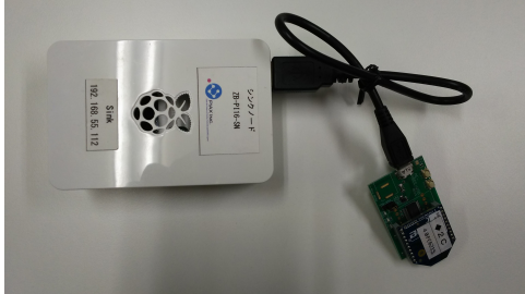
Fig. 16 Implemented sink node and cluster head node.
