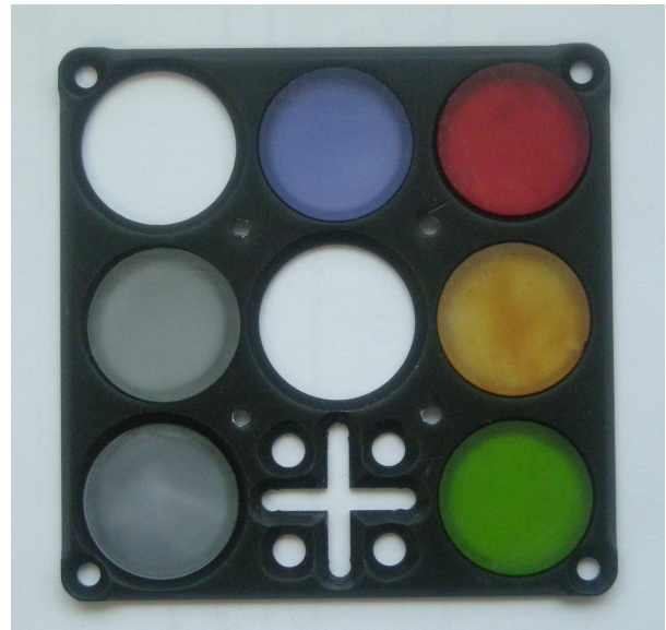
Figure 6. An earlier version of the PCT top retaining plate (inverted) with example stained glass wafers.
