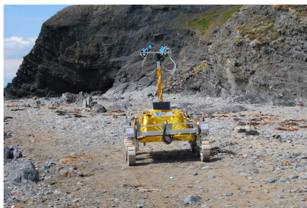
Figure 1. EADS Astrium Bridget rover with the AU PanCam Emulator (AUPE) undergoing field trial experiments at Clarach Bay beach, Ceredigion, UK.
