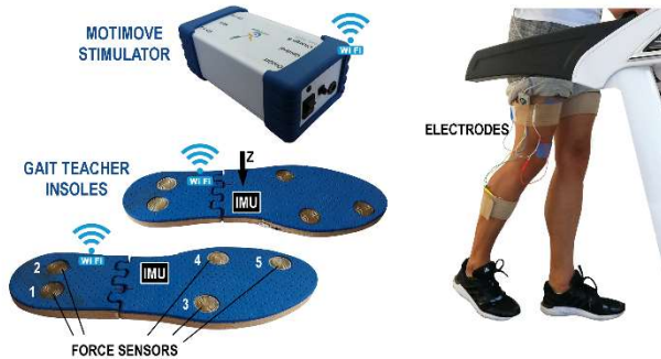
Fig. 2: "Gait teacher" insoles with five robust pressure sensors and one inertial measurement unit (IMU) each, "MOTIMOVE" stimulator for surface activation of up to eight muscle groups and the sketch of the person with hemiplegia when assisted with the system and using the rolling walker.
