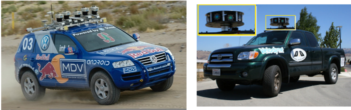
Figure 1. Stanley, the winner of the 2005 DARPA challenge equipped with five SICK LMS-291 2D LIDAR units and Hall brother's "Team DAD" truck equipped with their own 64-lasers spinning disc Velodyne 3D LIDAR (Source: DARPA)
