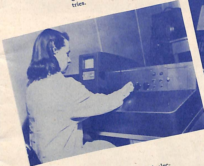
Console model of the RCA electron microscope enables photographic enlargement up to 100,000 diameters, depending on the subject matter.
