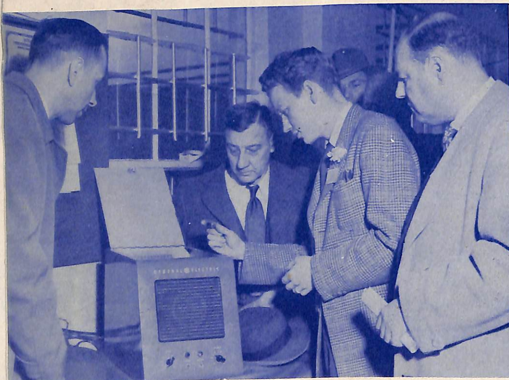
Close-up of GE high frequency FM emergency communications receiver used to pick up messages from transmitter in auto 50 miles away.
