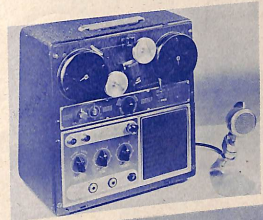
Wire recorder, will record 66 minutes continuously. Used by Army in many
