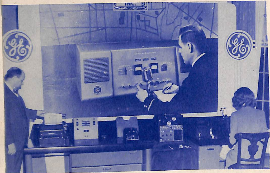
Complete radiotype automatic two-way station equipment in operation. A. C. Holt of I. B. M. Radiotype Division, inspects message as it comes off the radio.
