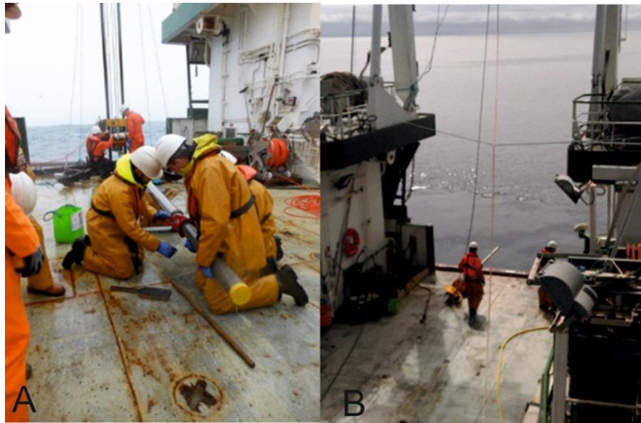
Figure 3.3: An example of the deck crew (A) bringing in a vibrocore after coring the Celtic shelf, on the GATEWAYS2 cruise, and (B) preparing for piston coring on the CE16010 cruise, on board the RV Celtic Explorer.
