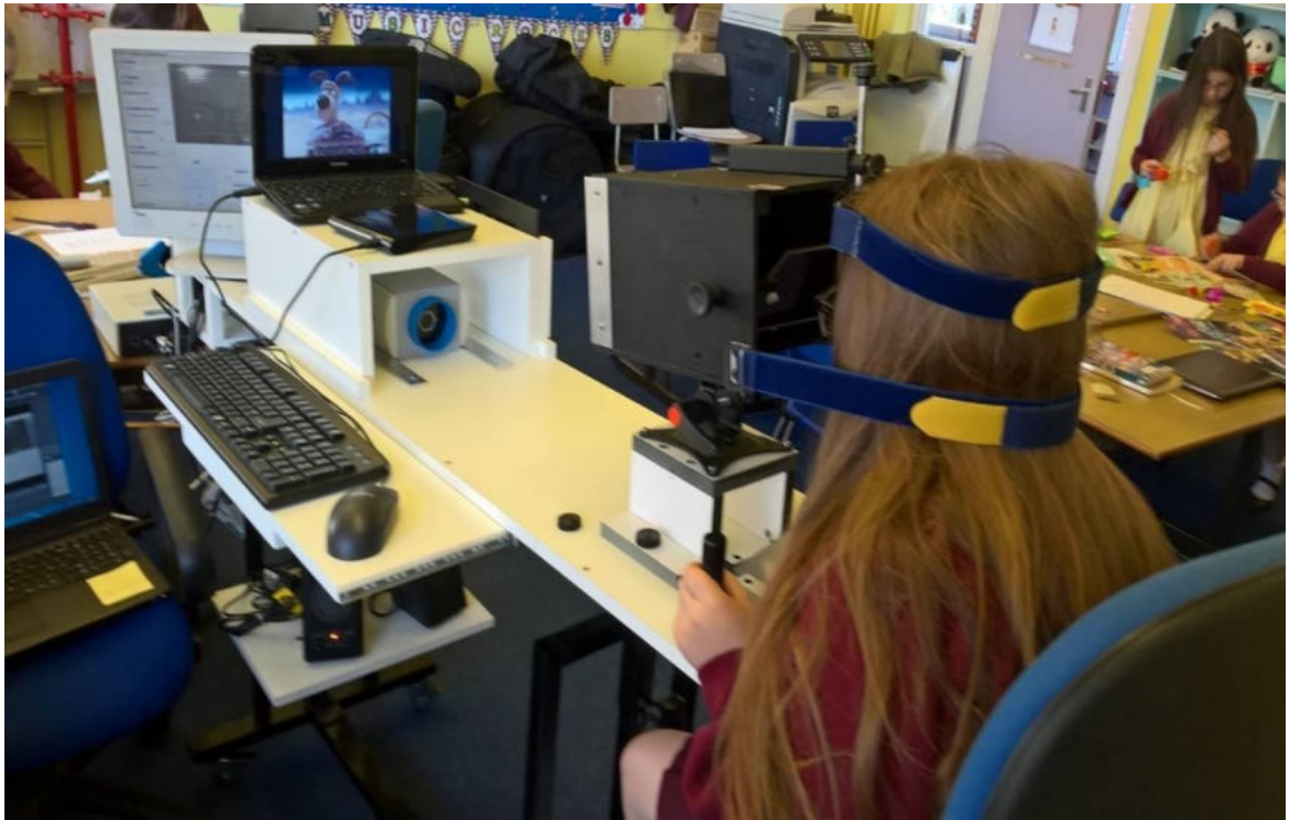
Figure 3.5.1 Image of the PowerRef 3™ set-up, showing a participant engaged in the movie task. The PowerRef 3™ was positioned 1m from the participant and connected to a computer (desktop) monitor. The participant's head was stabilised using two Velcro straps.
