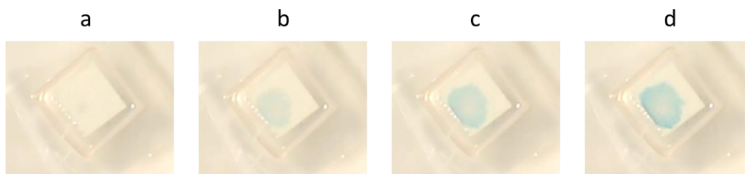
Figure 3.25 Digital photographs of paper backplates attached to 350 \mu\text{m} MN pierced through parafilm and placed on 10 mM glucose solutions (a) initial wetting of backplate (b) 20 s after wetting (c) 40s after wetting (d) 60s after wetting
