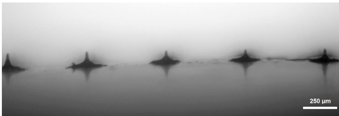
Figure 3.8 Optical microscope image of 350 \mu\text{m} MN tips pierced through a single layer of parafilm. Scale bar is 250 \mu\text{m}
