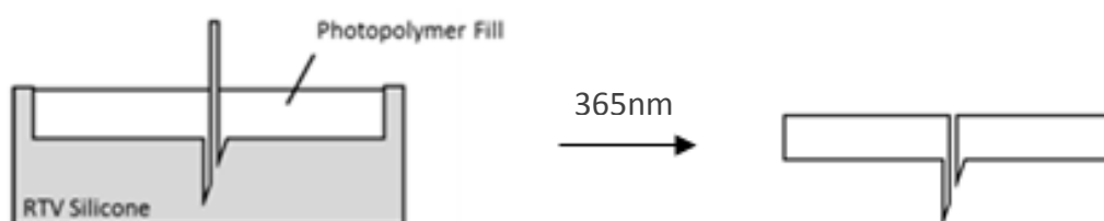
Figure 4.5 Schematic of hollow MN production. Silicone mould is filled with 150 \mu\text{L} of photopolymer mix before irradiation with UV light. Hollow polymer MN is then removed from mould.
