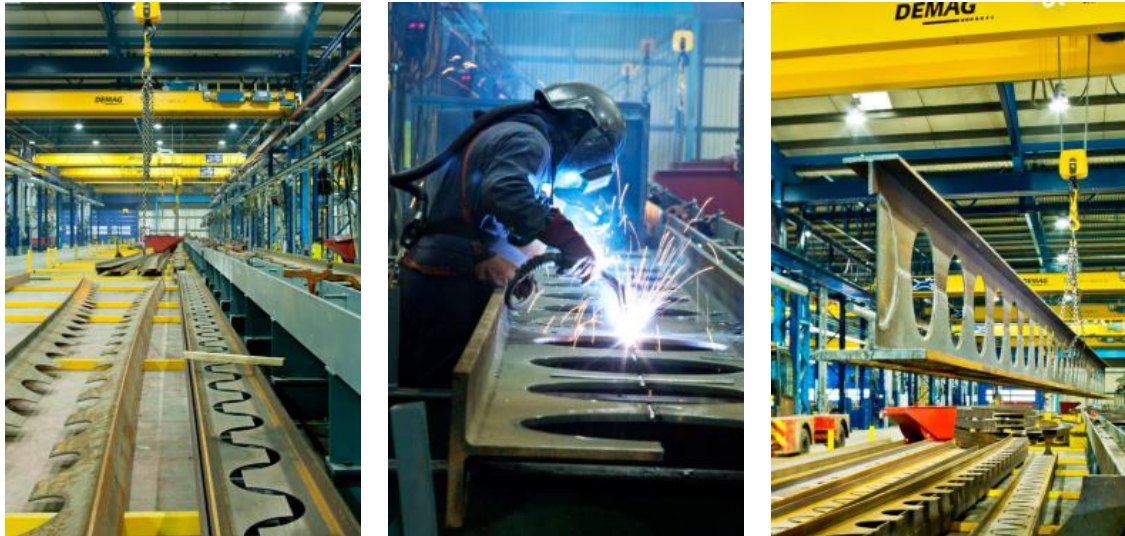
Figure 2.5-1 Fabrication of perforated beams [24]
