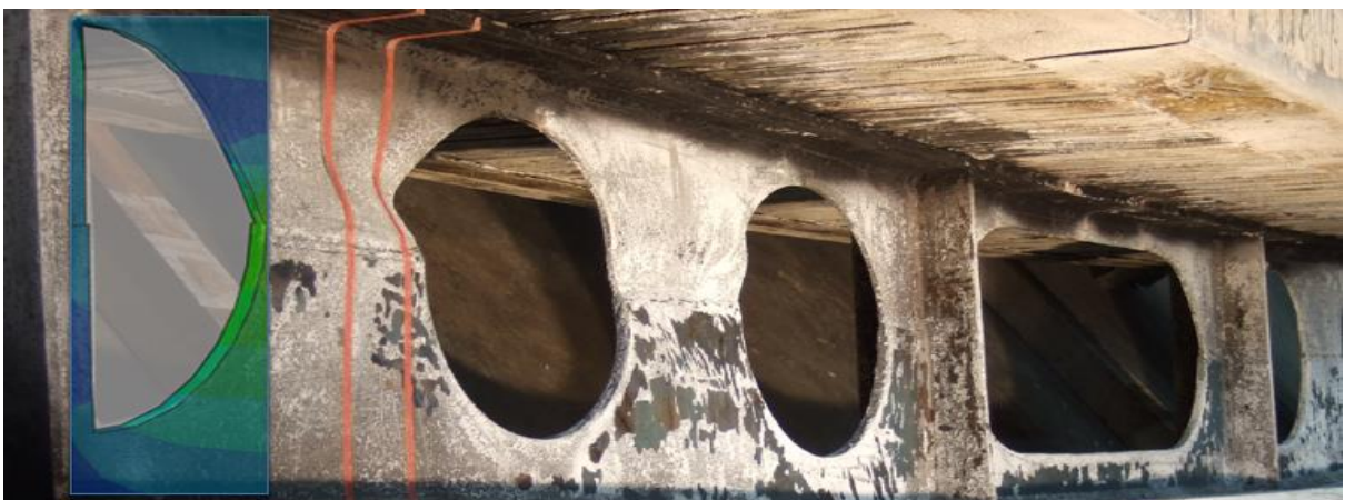
c) Deformed Beam 1, FEA and experiment
