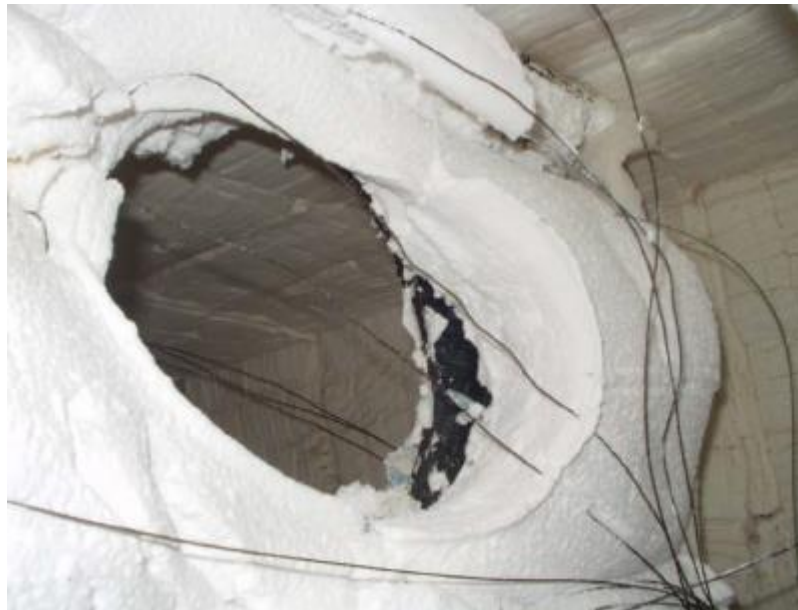
Figure 2.6-1 Intumescent pull back effect [30]
