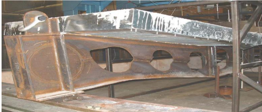
a) Deformed shape of beam with excessive failure after deformation - Test
