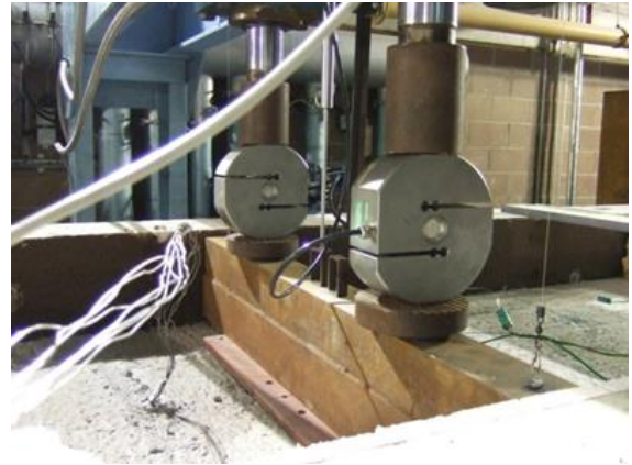
b) Hydraulic jack, spreader beam and LDVT
