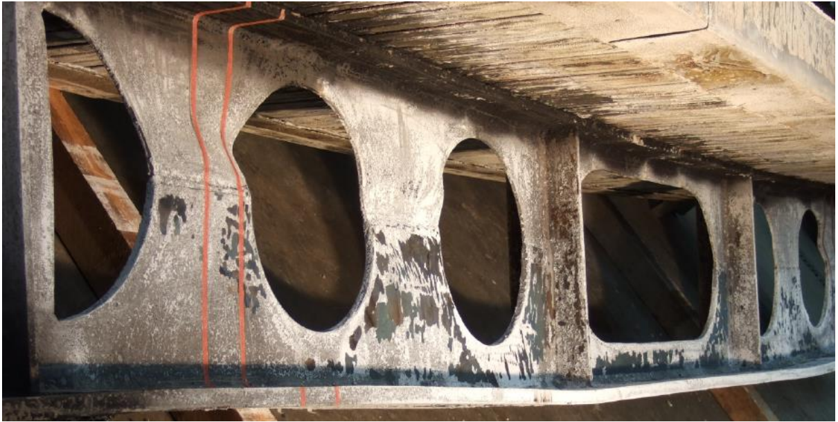
a) Deformed Beam 1, experiment
