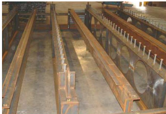
Figure 4.3-2 High density welded shear studs [51]
