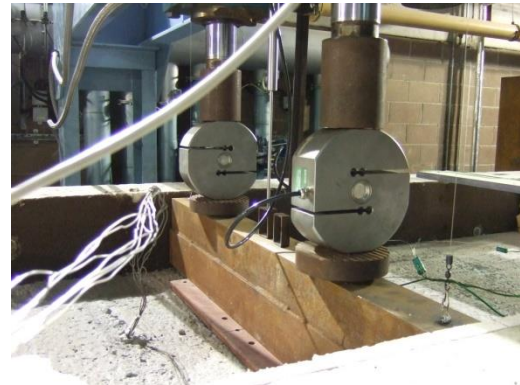
b) Hydraulic jack, distribution beam and LDVT
