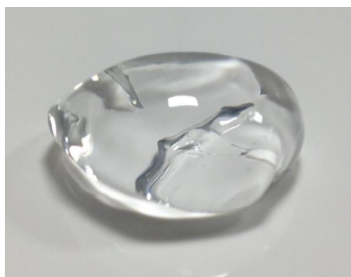
Figure 2.8 Picture of a sample of a PVA (6.0 % w/w)–borate (2.0 % w/w) hydrogel at room temperature, manufactured as described in section 2.4.1.
