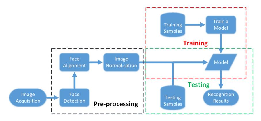
Fig. 1. The basic framework of a face recognition system.
