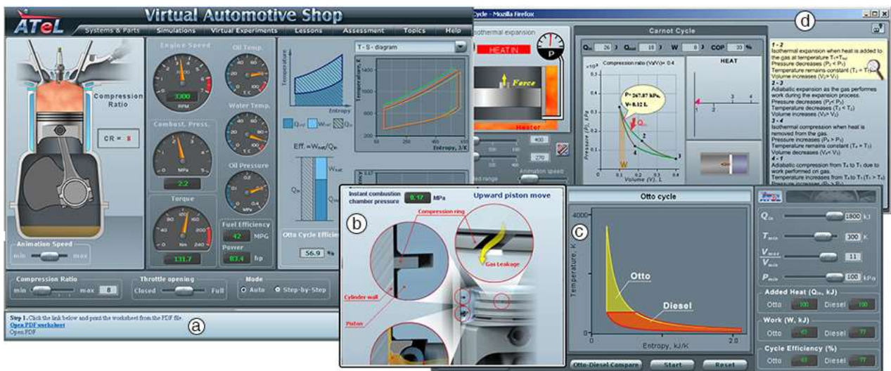
Figure 4. The virtual experiment “Influence of Compression Ratio on Engine Operation Cycle” performed at the v-Lab “Internal Combustion Engine Design and Operation” (a). Gauges in the middle panel display the major engine parameters such as fuel consumption, torque, power, rotation speed, pressure, oil and water temperatures and oil pressure. The right panel dynamically presents thermodynamic diagrams of engine operation. The screenshot (b) shows a fragment of the virtual experiment that enables automotive engineers and technicians, as well as car drivers who are eager to know more about vehicle maintenance, to explore how piston ring wear impacts engine performance and efficiency. The v-Lab “Thermodynamic Cycles” allows the student to explore in detail the Carnot cycle (c), Otto cycle and Diesel cycles, as well as to compare them with each other (d).
