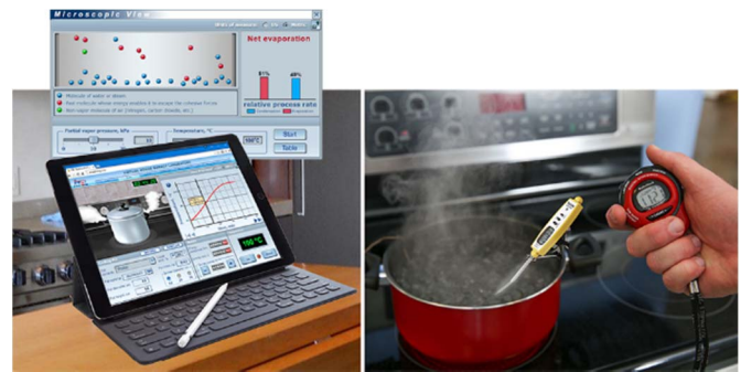
Fig. 5. Blended experiment in which students measure time and energy needed to boil a type of liquid (right) using cooking pots of different sizes, shapes, and made of various materials. In the course of the experiment the ratio of diameters of pots and cooktop burners could be changed as well. The identical experiment is performed online in the v-EEH kitchen (left). Auxiliary simulation (top left) synchronized with the virtual pot dynamically visualizes processes occurring at the microscopic level.
