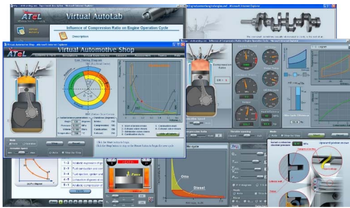
Fig. 8. The simulation, shown in the middle left, dynamically imitates the operation of an internal combustion engine that is linked and synchronized with a Cam Timing Diagram and the chart displaying the Otto cycle (right panel). The student is able to investigate the connections between events taking place in the cylinder and parameter changes at any stage of the cycle. This helps students better appreciate Otto cycle by visualizing how thermodynamic processes occur in an engine. Using the simulation presented in the middle right, students can explore how engine compression and throttle opening affect operating cycle and the influence on engine performance and efficiency. Digital and analog gauges display the major process parameters such as fuel efficiency, torque, power, rotation speed, pressure, oil and water temperatures and oil pressure. The bottom right screenshot shows a fragment of the simulation that was designed to help automotive engineers and technicians, as well as drivers who are eager to know more about vehicle maintenance, explore how piston rings wear impacts engine performance and operation cycle. The simulation shown in the bottom center enable to visually compare different thermodynamics cycles (Otto, Diesel, Rankine, and Carnot) and study their dependency on various parameters. Virtual experiments combine simulations with educational resources and assessments (bottom left).
