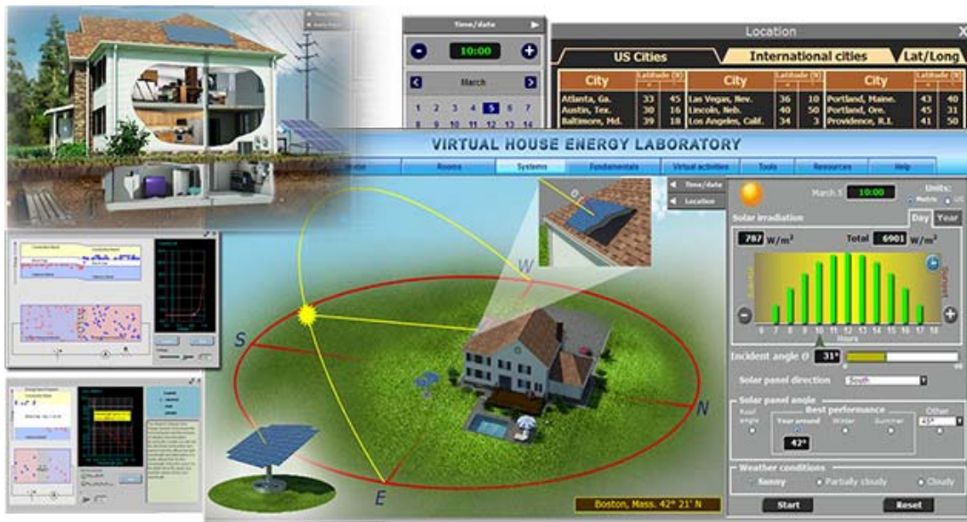
Fig. 3. The set of simulations modeling solar heating and photo-voltaic (PV) systems. Students can change many parameters of the simulations and explore how solar irradiation and efficiency of the systems depends on seasons and daytime (a), geographical location (b), house and panel orientation, weather conditions and some other factors. It is possible to switch between fixed tilt and auto (sun-tracking) PV systems. Auxiliary simulations (shown in the left) imitate the basic processes in semiconductors responsible for converting, light energy into electricity, which enable students to study photovoltaic effect in semiconductors and explore factors affecting the efficiency of PV panels.
