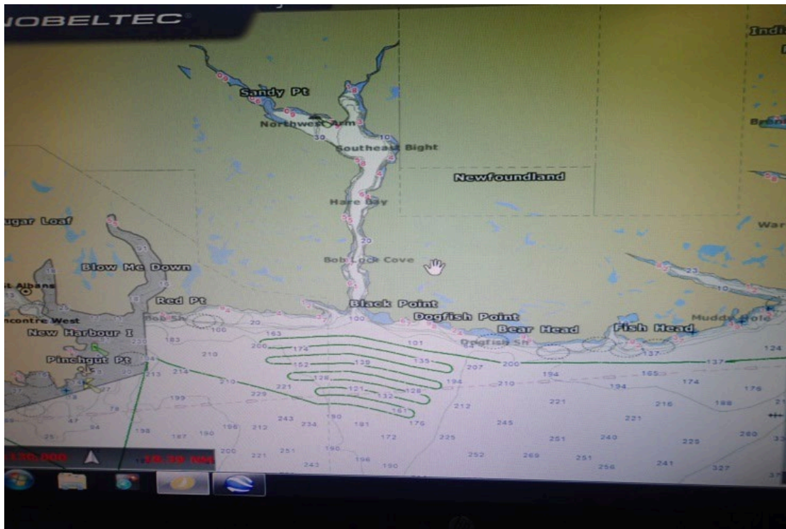
Figure 6. Showing the ship tracklines of the multibeam and seismic survey conducted across the mouth of Hare Bay.
