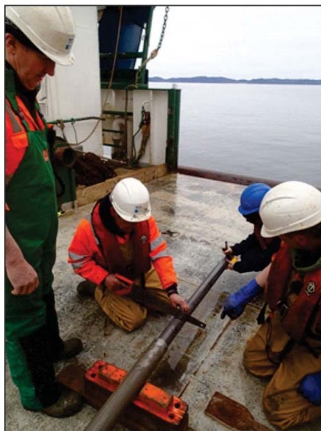
Plate 3. Core liner was measured into 1 m segments and cut with a handsaw. Caps were placed on the ends of the core after cutting.
