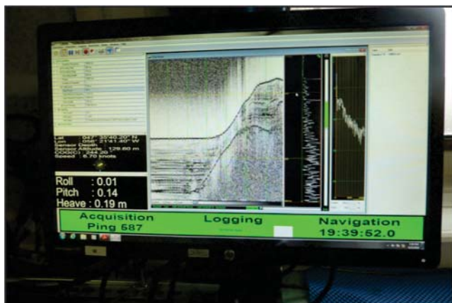
Plate 6. Screen shot of a seismic profile showing the quality of the data. Note the various horizons that capture the sedimentary architecture of the seabed along the survey path.
