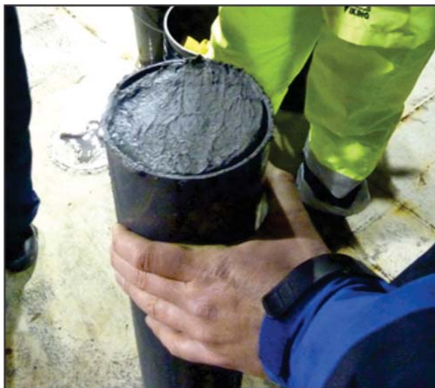
Plate 5. Grey mud inside a section of core liner recovered using the vibro-corer in Bay d'Espoir.
