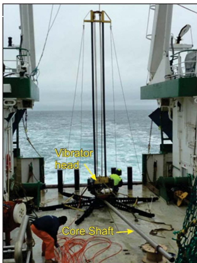
Plate 1. Vibro-corer used during the NISS survey. The vibrator head (yellow) is located toward the base of the corer whereas the grey core barrel extends from the corer toward the bottom right for retrieval of core. The vibrating head moves to the top of the corer once the core barrel is brought to an upright position.
