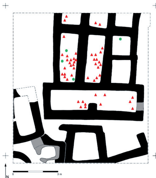
Figure 12 Tell Sabi Abyad. Distribution of roof material fragments in the burnt building V6. Clay roof fragments with reed imprints (red triangle), wood remains (green circle).
