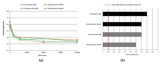
**Figure 11.** (a) Texture depth development up to 100,000 wheel-passes; (b) texture depth ranking after 100,000 wheel-passes (Ulster University data).
