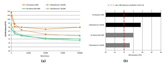
**Figure 10.** (a) Skid resistance development up to 100,000 wheel-passes; (b) skid resistance ranking after 100,000 wheel-passes (Ulster University data).
