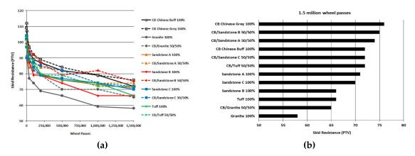
**Figure 3.** (a) Skid resistance development up to 1.5 million wheel-passes; (b) skid resistance ranking after 1.5 million wheel-passes (Aetec data).
