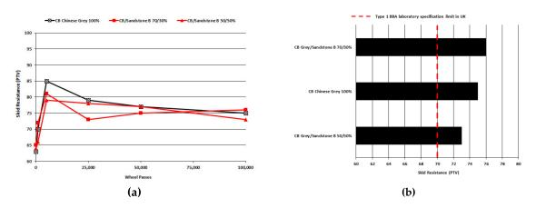
**Figure 6.** (a) Skid resistance development up to 100,000 wheel-passes; (b) Skid resistance ranking after 100,000 wheel-passes (Ulster University data).
