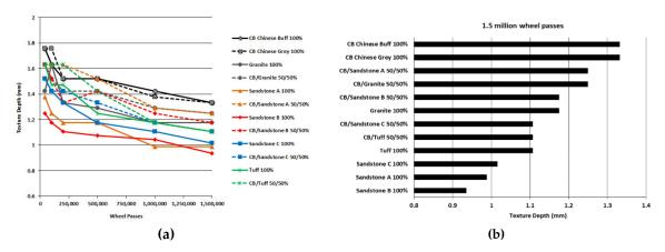
**Figure 4.** (a) Texture depth development up to 1.5 million wheel-passes; (b) Texture depth ranking after 1.5 million wheel-passes (Aetec data).
