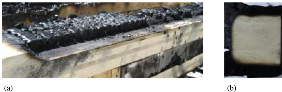
Fig. 2. Charcoal protective layer of (a) CLT panel [2] and (b) solid timber beam [5].
