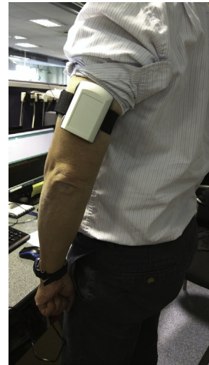
Fig. 15. Prototype of LUA wearable band monitoring device (WASTCARd Project), for long-term heart rhythm monitoring.
