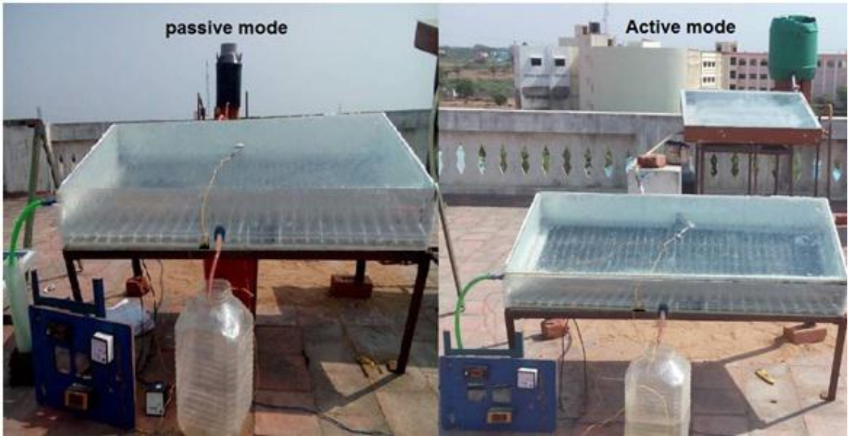
Fig. 2 Experimental arrangement of passive and active ISPB still
