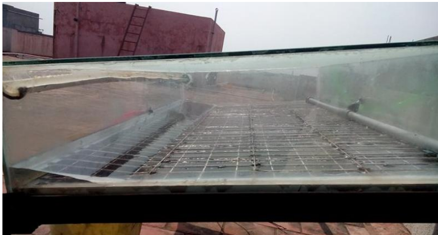
Fig. 3 Water flowing arrangements within the ISPB still.
