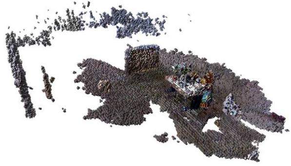
Fig.13 The simulation results of “freiburg2-desk” based on the proposed method: (a) dense point cloud map; (b) octomap map
