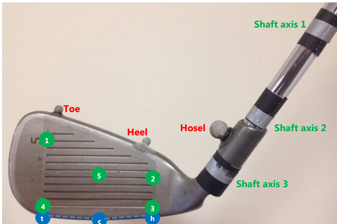
Figure 2: Marker placement on clubhead and hosel.
