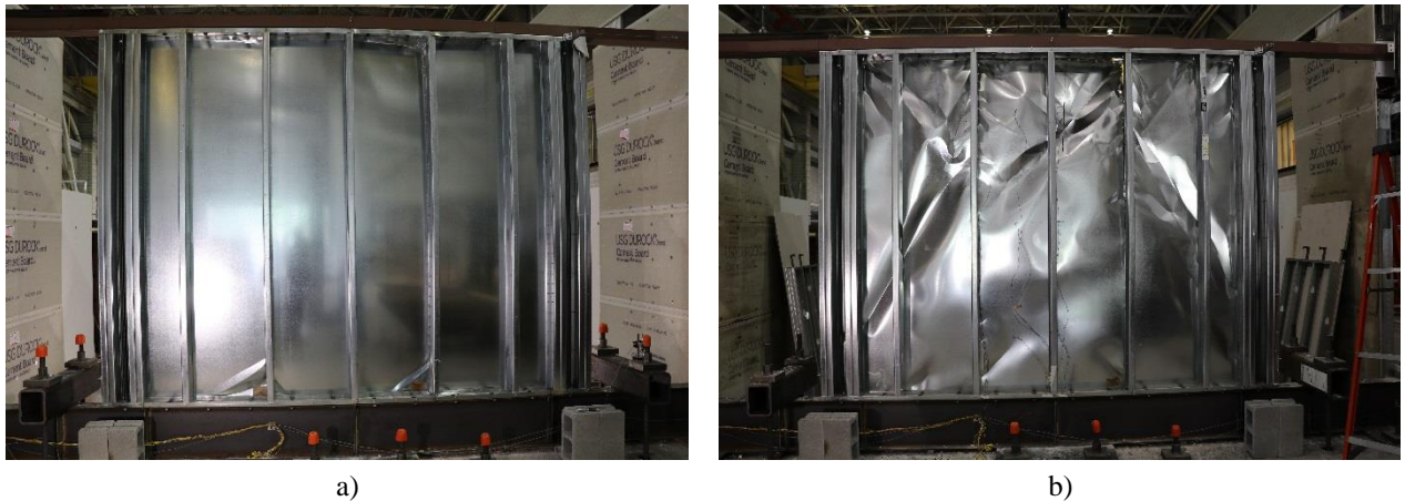
Fig. 4. Photograph of back of sheathed side of wall with the nonstructural gypsum removed after mechanical loading to failure: a) Unburned wall after cycling (local buckling); b) Cycling after burning (global buckling)
