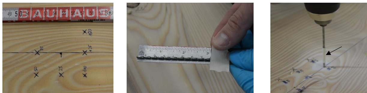
Figure 4: Drilling procedure: grid marking (left), measuring the depth (centre), drilling with depth-marker (right)
