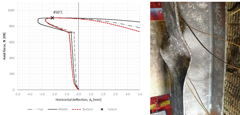
Figure 3 Load-deflection response (left) and post-failure buckling response (right) for Test 3 (concentric loading)
