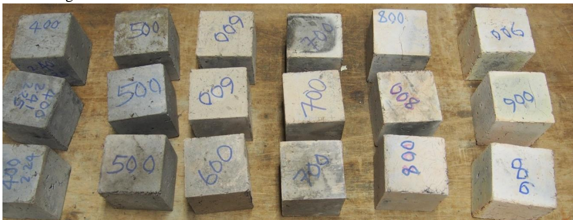
Figure 2. 100 mm cube specimens after being heated at various temperatures
