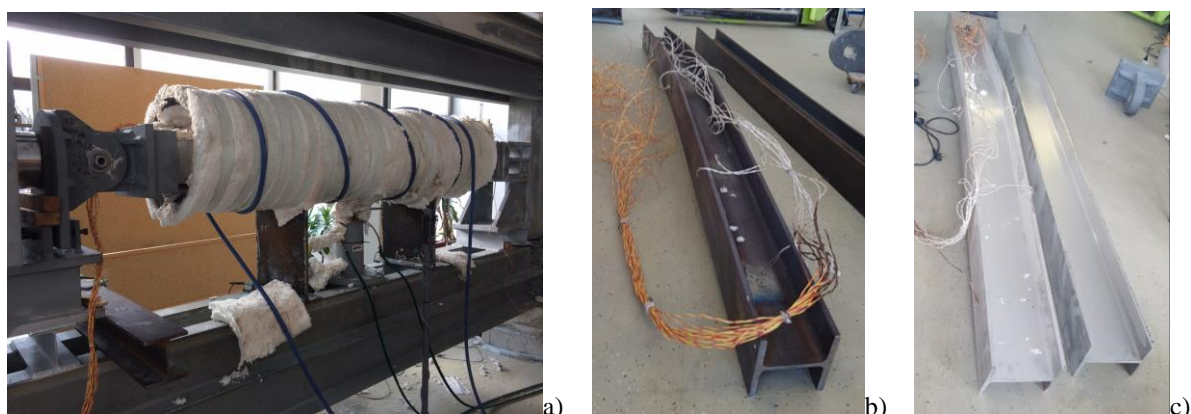
Fig. 1. a) Test setup for aluminium columns; b) steel column; c) aluminium column
