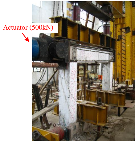
Fig. 3 Overview of reversed cyclic loading test setup
