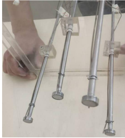
Fig. 2. Placement of thermocouples and pressure gauges
