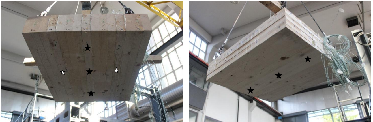
Figure 1: STP (left) and CLT (right) specimens, fire exposure on bottom surface, with indicated positions of the measurement stations (stars)
