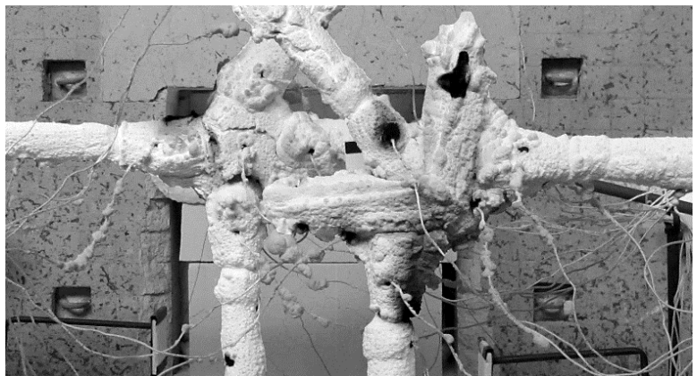
Fig. 3. Specimens after the fire test (DFT 3.5 mm)
