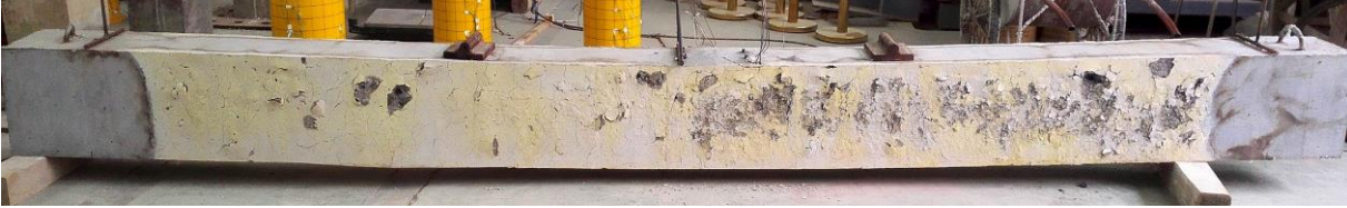
Fig. 3. Failure mode of the SRU beam
