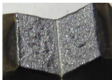
BM specimen subjected to 700°C heating
