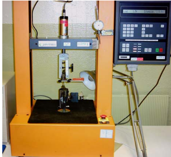
Figure 2. Machine (Lloyd L-1000 R) for measuring tensile strength of the cotton strips.
