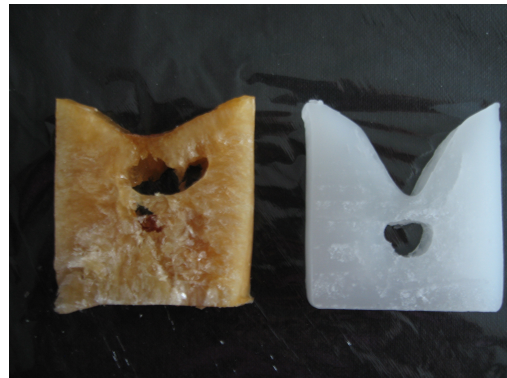
Figure 5 The porosity at the centre of the bulk for PCM Waksol A and RT35 with a -25^{\circ}\text{C} solidification temperature.
