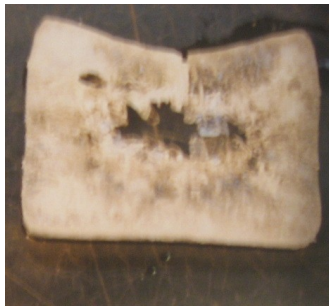
Figure 3 The porosity at the centre of the bulk PCM RT25.
