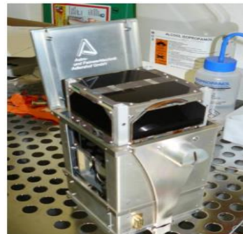
Figure 7: SwissCube FM in its Single Pod Deployer. Source: Astro und Feinwerktechnik AG [30]
