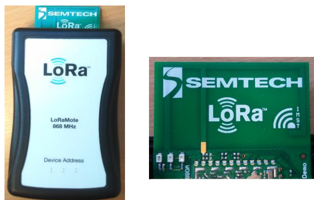
Fig. 1. Semtech LoRamote device used for testing including the inverted-F antenna
