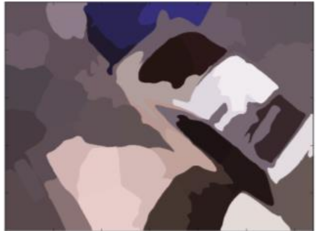
Figure 3. SLIC superpixel segmentation of RGB image with average RGB values within each of the 50 superpixel regions computed.
