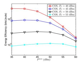
Fig. 4. Effect of circuitry power consumption on the energy efficiency.
