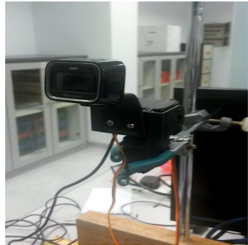
Fig. 2. The Microsoft LifeCam HD-5000 Camera mounted on 2 servomotors.
