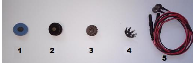
Figure 4. Dry electrodes used for the measurements: 1) AgCl stud, 2) Iron, 3) Polyurethane multipin-A, 4) Polyurethane multipin-B, 5) Silver disc.
