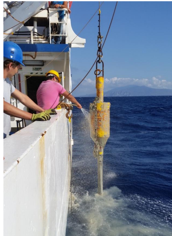
Fig. 4.7 (right) Recovery of gravity corer. The mud all over the barrel and weight of the corer is an indication of complete penetration.
