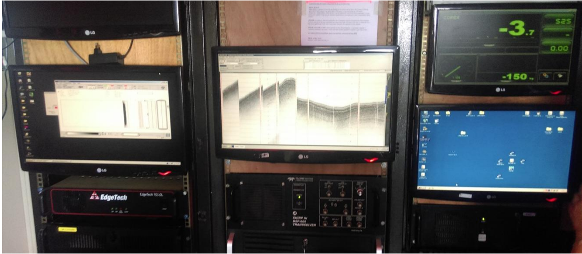
Fig. 4.3 Seismic acquisition station. The centre screen shows the CHIRP data being acquired. The scientific staff on geophysical watch would take care of data quality, changes in delay and of initial interpretation of data in order to select the optimal locations for coring.
