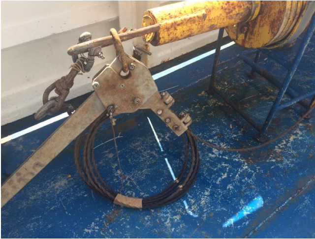
Fig. 4.6 (top) Particular of the trigger system for gravity corer.
