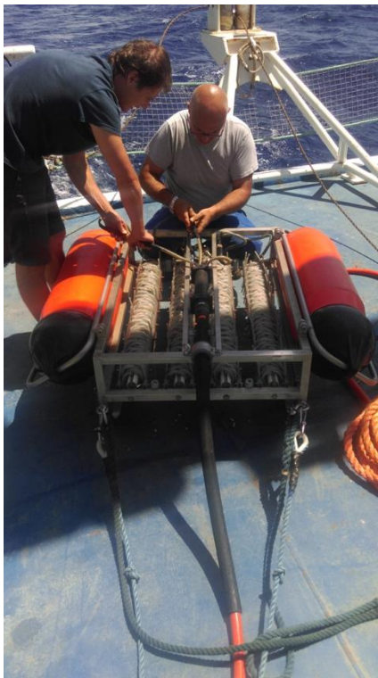
Fig. 4.4 The ship technicians getting the Geo-Source 1500 sparker ready for deployment.
