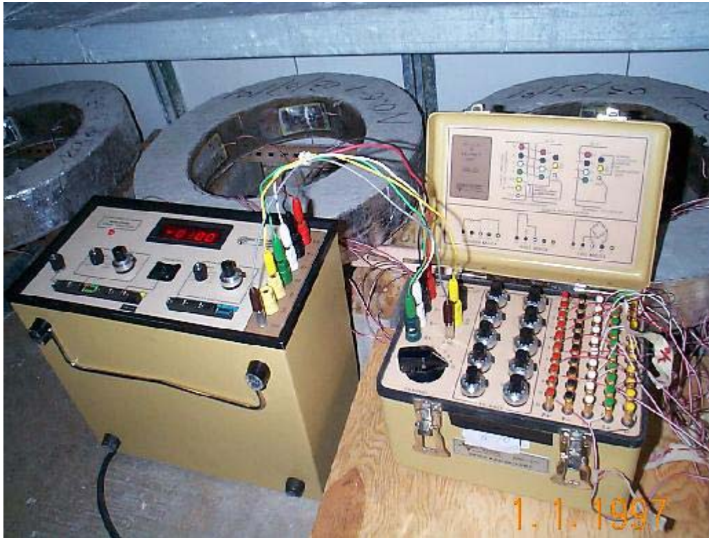
Figure 5.38: Set-up of Concrete Ring Test
