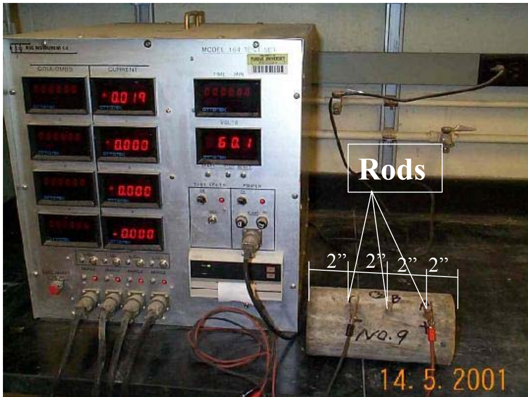
Figure 5.27: Set-up of DC Electrical Resistance Test
