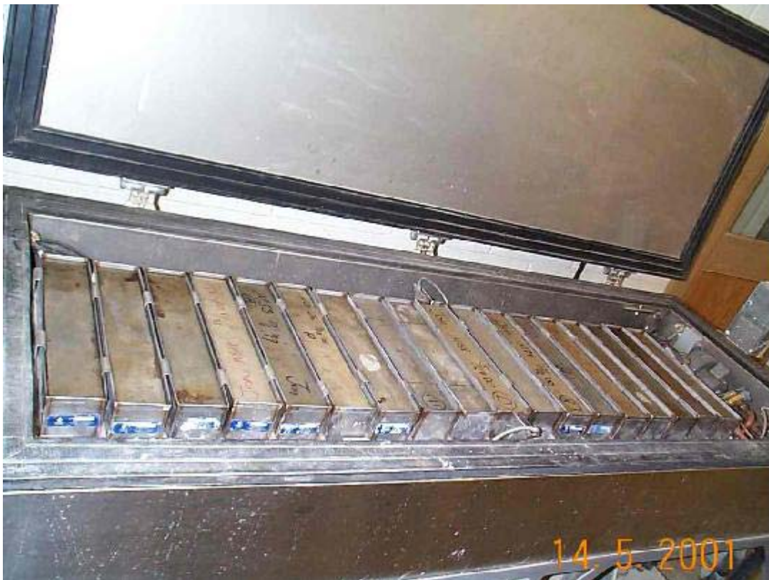
Figure 5.21: Set-up of Freezing and Thawing Test
