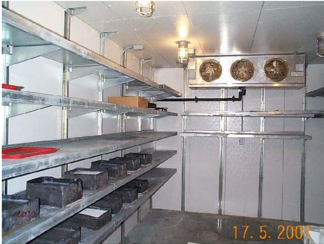
Figure 5.23: Set-up of the Test for Scaling Resistance to Deicing Salts
