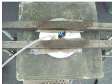
(b) The test head without the guard ring
