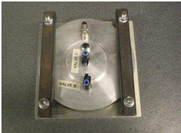
1 2 (a) The test head with the guard ring
