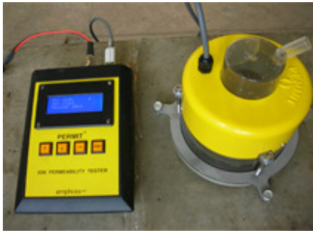
Figure 7. Permit Ion Migration Test
