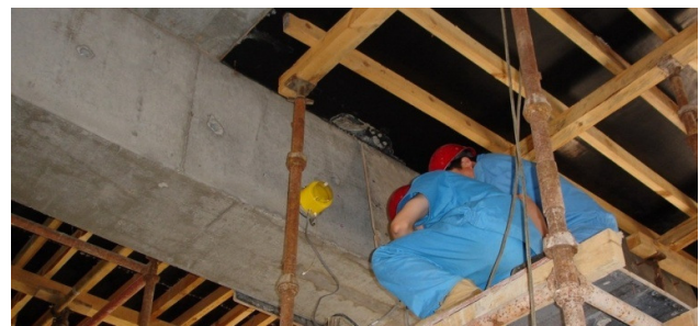
Figure 6. Autoclam used to test concrete in Bird Nest National Stadium, Beijing, China
