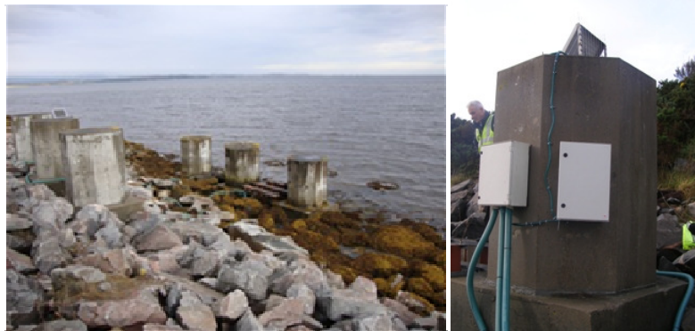
Figure 10. Exposure site in Scotland with remote data collection and solar power units
