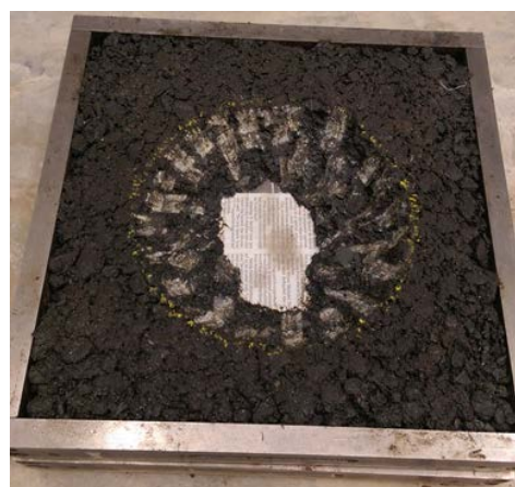
Figure 1. Simulated pothole for geopolymer repair material investigation.
