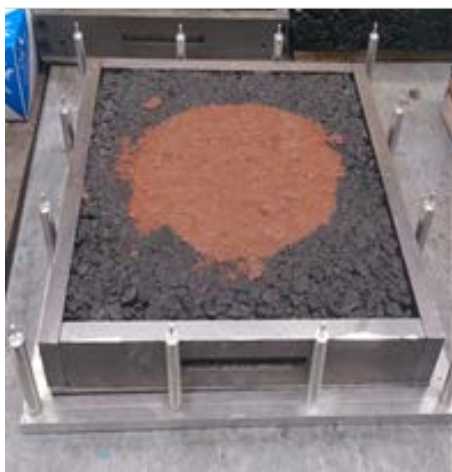
Figure 7. Geopolymer pothole repair material after simulated wearing.
