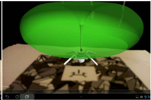
Fig. 11.12. Spider antenna with radiation pattern in 3D.
