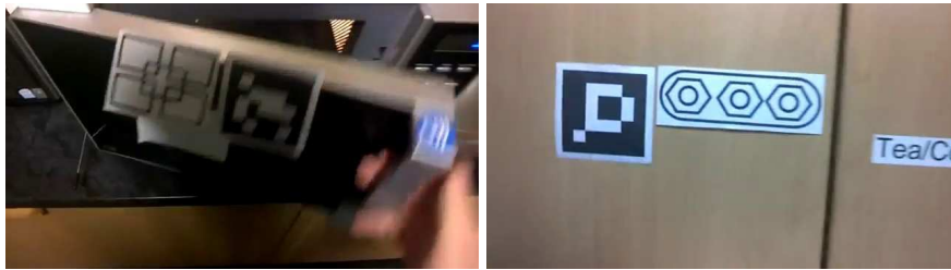
Figure 6. Frames from the wearable vision sensor showing first person view of interactions with objects. A) Low brightness and high motion blur situation. B) High brightness and low motion blur situation.
