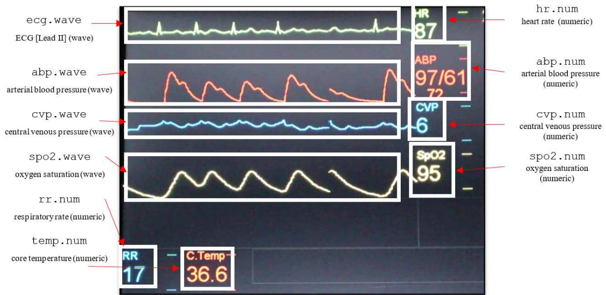
Figure 2. Simulated Vital Signs Screen with Eye Tracking Areas of Interest with Variable Names Highlighted
