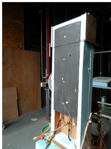
Figure 2: Prototype HyPVT unit (V1 09/03 without PV panels) ready for testing
