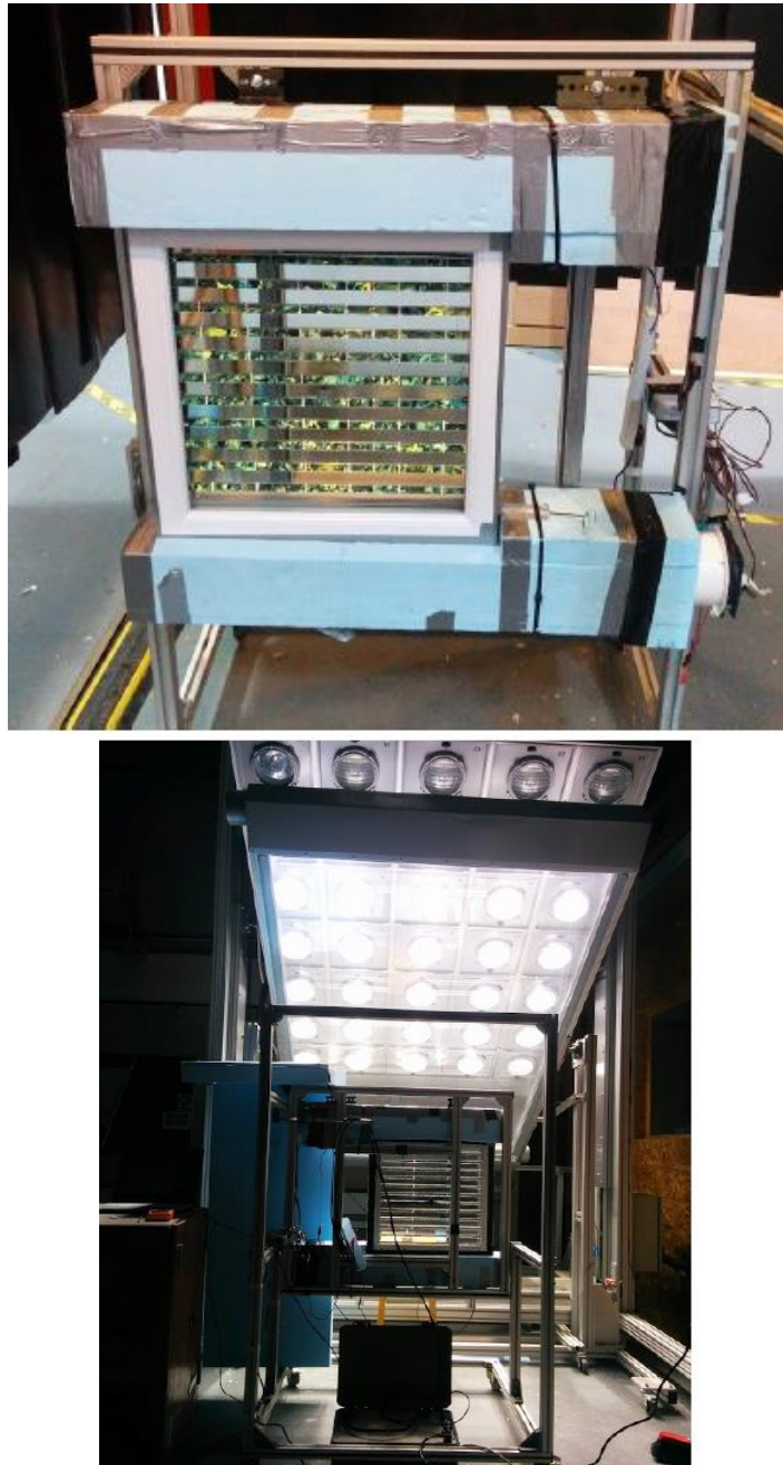
Figure 4. Front view of the experimental CoPVTG prototype (left) and rear view (right) placed under the solar simulator
