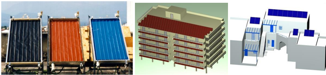
Fig. 2 Tested colored collectors and application examples on a building roofs
