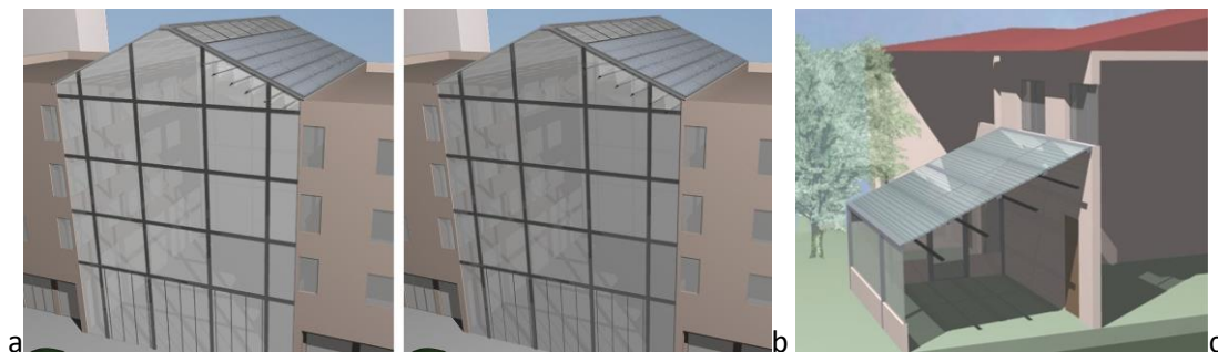
Fig. 16 Example of Fresnel lens integration on building atrium (a, b) and sunspace (c)
