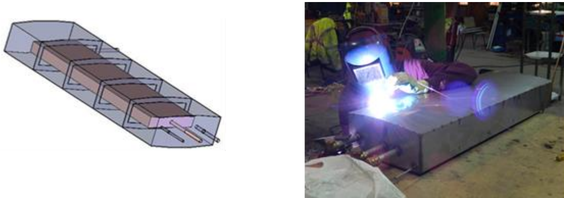
Figure 1: Detail of the small scale laboratory prototype HyPV/T unit and its final welding and assembly
