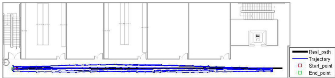
Fig. 5. Schematic diagram of pedestrian horizontal position with 15D Kalman filter state model.
