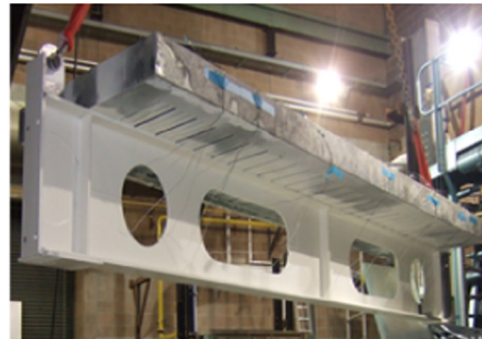
Fig. 1. Steel cellular beams with different opening shapes.
