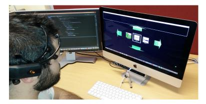
**Fig. 2.** A subject enacting Task 1 and operating the IGUI while using the EyeTribe Tracker and Emotiv EPOC as collaborative input modalities. The subject has successfully executed a right command thus scrolling the IGUIs menu from the *Back Garden* icon to the *Bathroom* icon.
